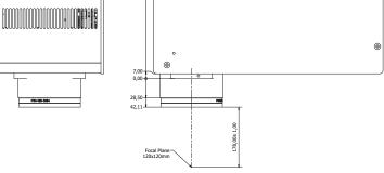
Dimensions are referred to F.L. 160 mm, objective diameter 85 mm. Other differents Focal Lenght objective are available upon request.
